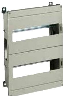
\*The DLM modular chassis consists of metal cut-out front panels which can clip on with any screws. Rigid structure made from galvanised steel. The depth of the chassis can be adjusted from 40 to 85 mm, between the rail and the front panel, allowing the installation of all types of devices. The enclosure can be equipped with accessories from the Spacial standard wall-mounting range.
